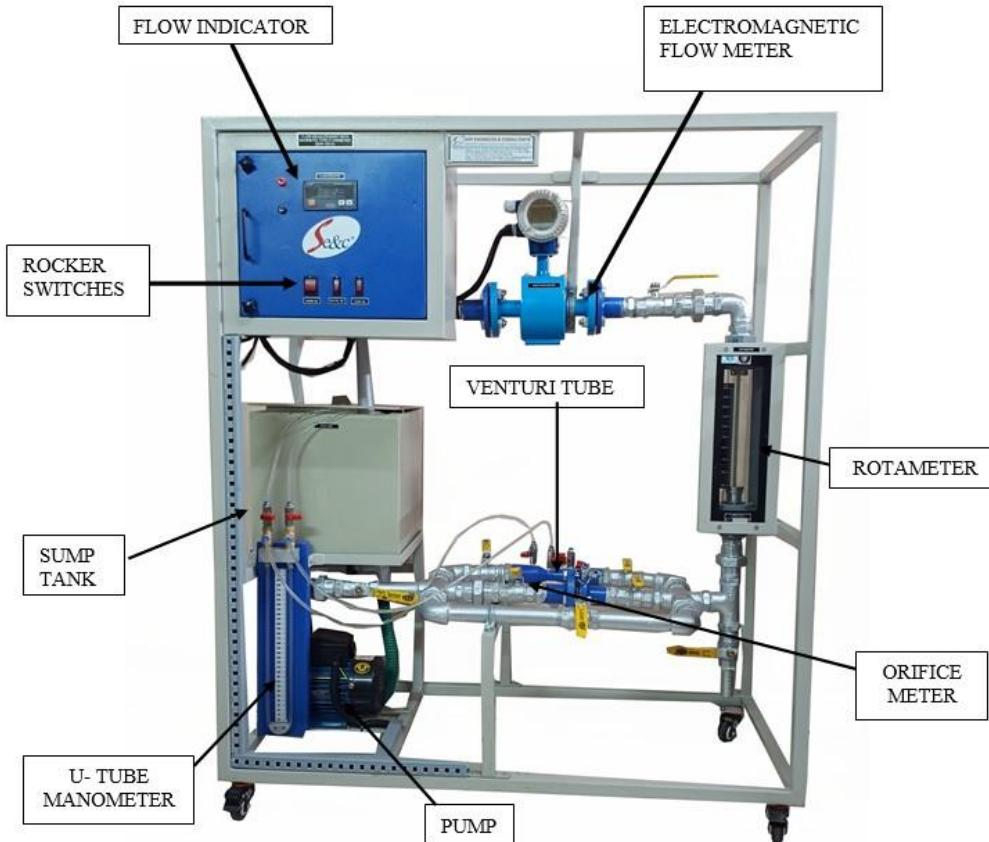
The **Setup for Calibration of Flow Sensor (SAP – 15D-II)** gives an idea regarding Flow Sensor & Flow Transmitter Principle. It outlines the procedure for calibration of flow Sensors/Transmitters.
